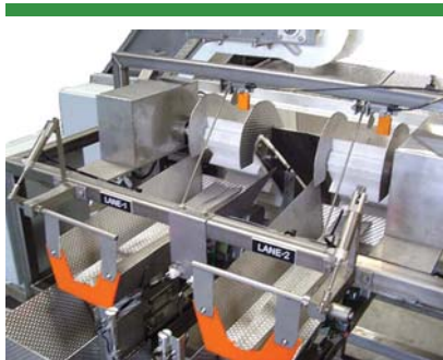
ME1095CVDX2 dual lane system with integrated cleat elevator for running pickled vegetables and frozen pastas in 3 lb portions at 14 to 24 cycles/minute.
